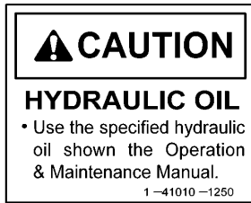
(19) Precautions for oil inside hydraulic tank (1-41010-1250)
